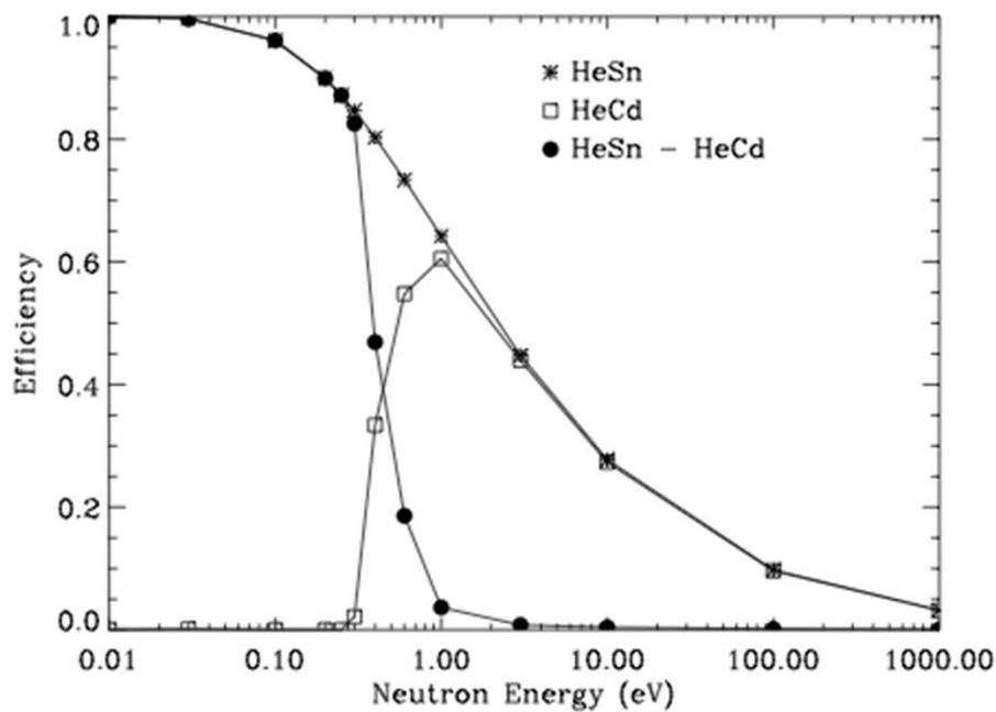
**Figure 11.** The response of the Sn- and Cd-covered  $^3\text{He}$  gas proportional counters calculated for neutrons incident at right angles to the counter symmetry axis.
