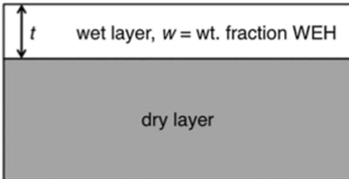
**Figure 1.** Layering stratigraphy being considered in this paper, where a top layer with thickness  $t$  and water equivalent hydrogen (WEH) abundance  $w$  overlies a completely dry layer.
