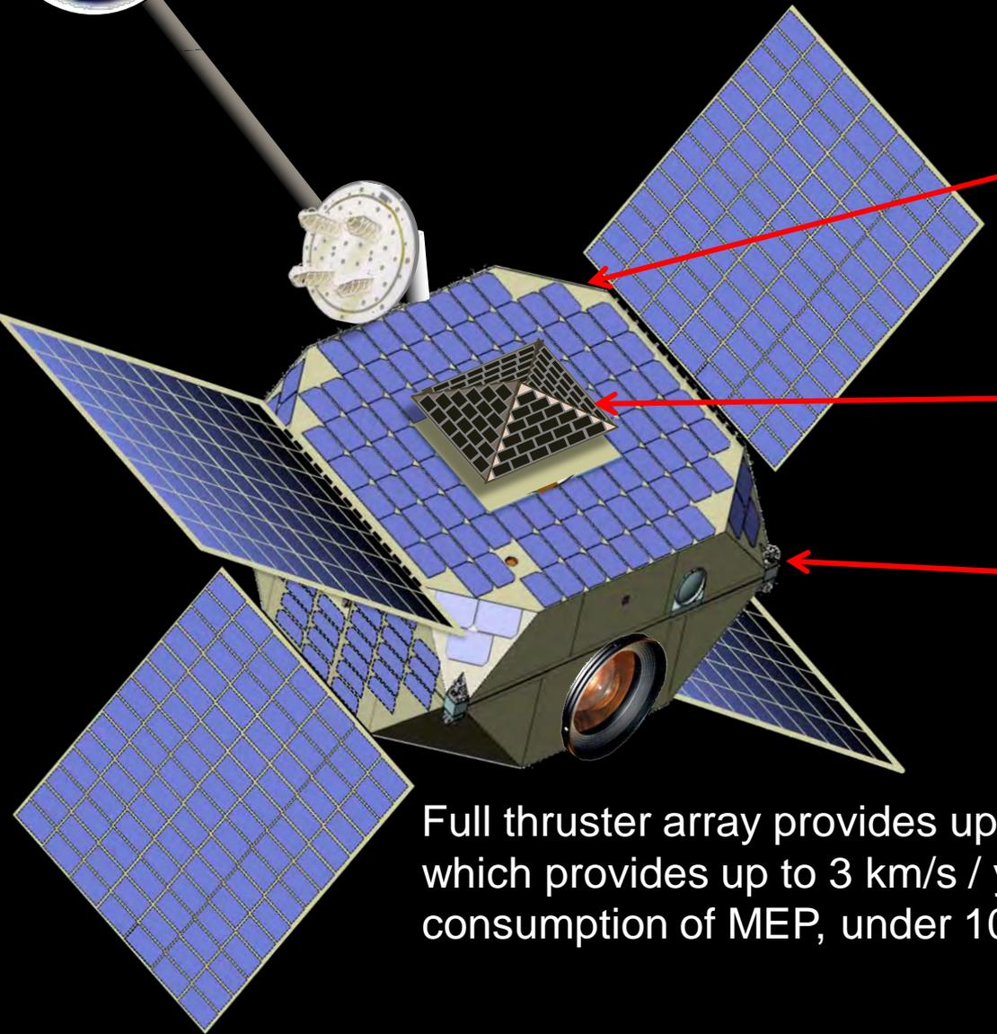
3D Array of MEP thrusters, arranged to allow removal of 3 dimensions of torque via bank-wise off-pulsing via Indium propellant heater cycling
