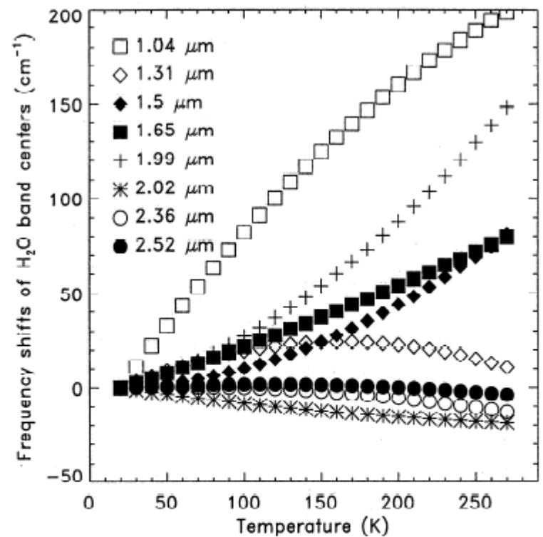
**Figure 5.** Examples of the temperature dependent shifts in frequency of several of our 12 well-constrained absorption bands, relative to the 20 K values which are tabulated in Table 1. These curves result from fitting Gaussians to the different components of the spectrum at each temperature, as described in the text.
