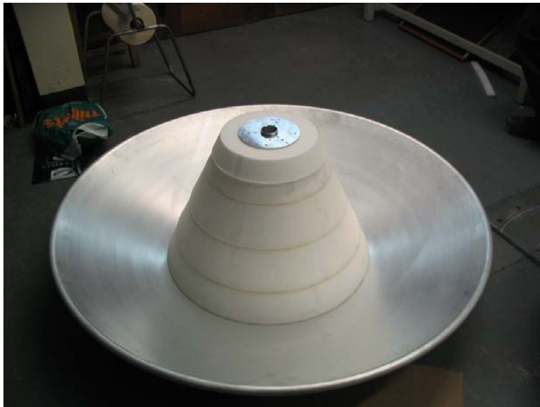
1.4m antenna with a foam mounted secondary built at Oxford
