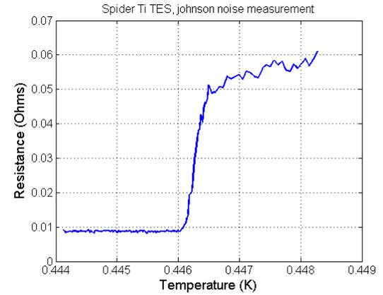
TES transition curve measured using Johnson noise.
