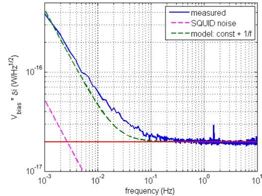
TES dark noise.  $NEP \sim 2 \times 10^{-17} \text{ W Hz}^{-1/2}$ , 1/f noise knee  $\sim 40\text{mHz}$
