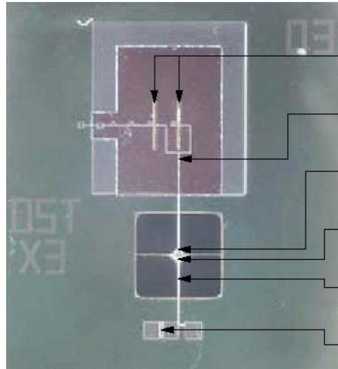
**Antenna-Coupled Superconducting Bolometer**
