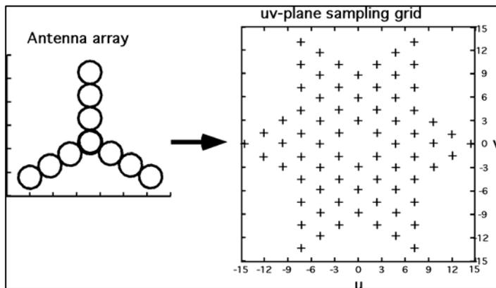
Receiver array → Resulting uv samples
