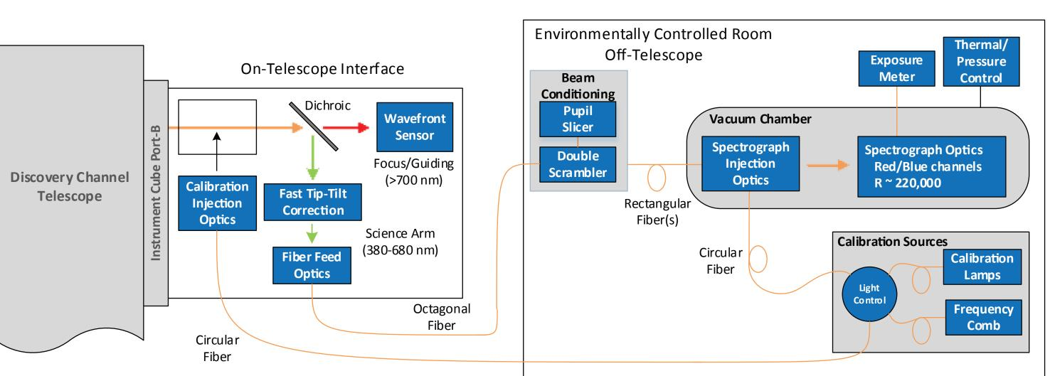
A schematic of the EXPRES instrument package is presented above, and consists of four subsystems:
