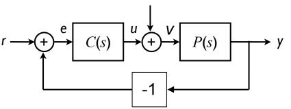
• Sensitivity function:  $S(\omega) = V(\omega)/D(\omega)$ ; want  $S(\omega) \ll 1$  for good performance
