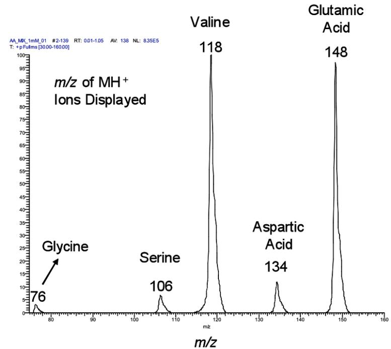
Mass spectrum of five amino acids produced via nanoelectrospray ionization of methanol/water solution
