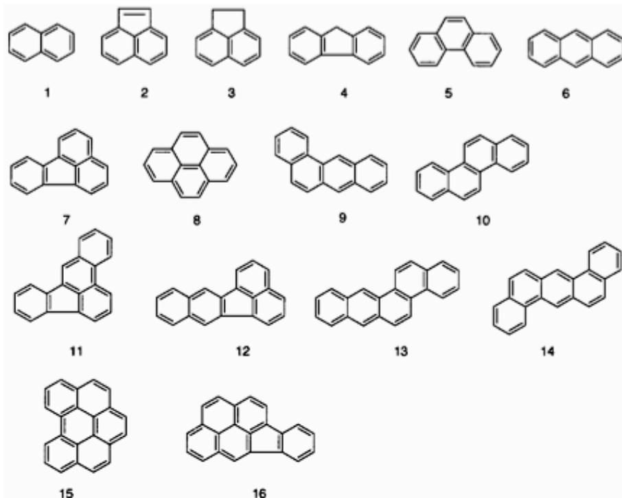
**Figure 4.** Structures of the PAHs: (1) naphthalene, (2) acenaphthalene, (3) acenaphthene, (4) fluorene, (5) phenanthrene, (6) anthracene, (7) fluoranthene, (8) pyrene, (9) benz[a]anthracene, (10) chrysene, (11) benz[b]fluoranthene, (12) benzo[k]fluoranthene, (13) benzo[a]pyrene, (14) dibenz[a,h]anthracene, (15) benzo[ghi]perylene, and (16) indeno[1,2,3-cd]pyrene.
