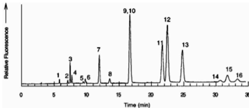
**Figure 5.** Electrochromatographic separation of 16 PAHs on the butyl stationary phase in 75:25 v/v acetonitrile/5 mM tris, pH 8, at field strength of 833 V/cm.
