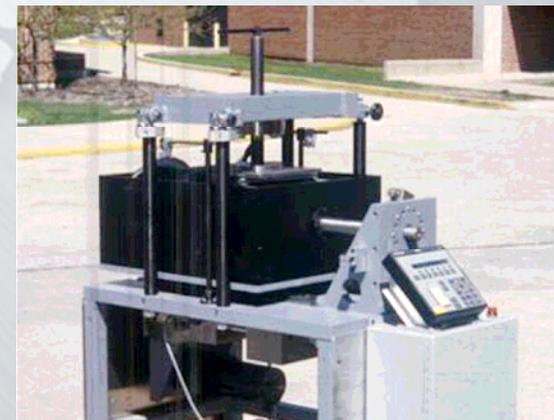
12"x12" Direct Shear Device at UIUC
