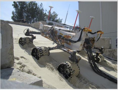
NASA's Mars Science Laboratory (MSL) Design/Test Model (DTM) in the sandy Mars Yard at JPL
