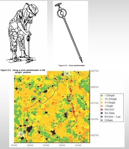
Map of HMMWV max speed based on cone index analysis
