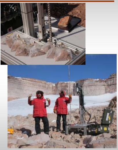
Honeybee Robotics IceBreaker rotary-percussive drill prototype being tested in Antarctice
