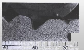
Figure 1.12: Soil flow under the action of grousers of a wheel in sand (Reprinted by permission of ISTVS from Wo et al., 1984)
