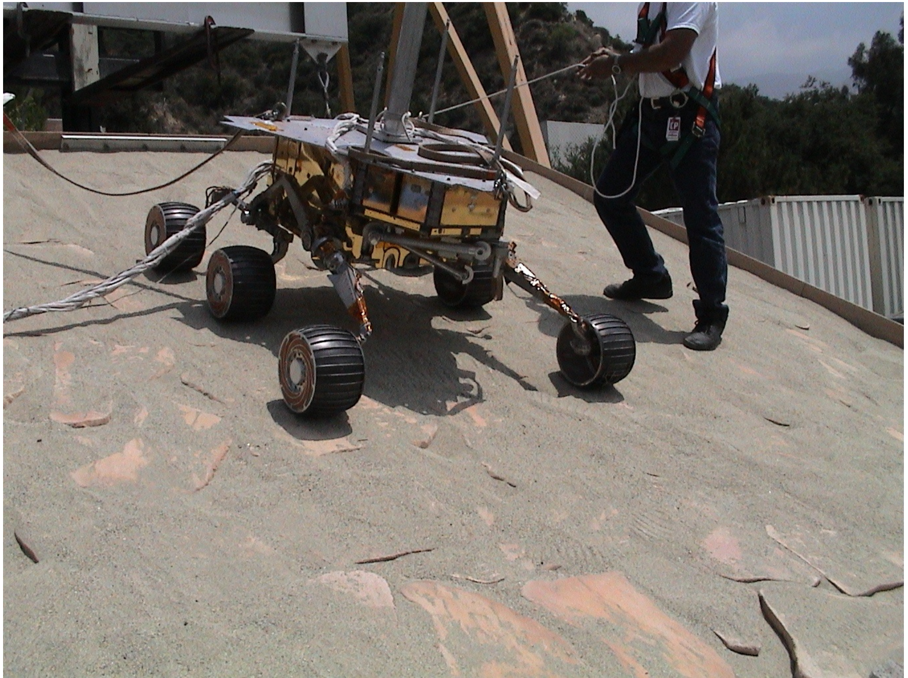
Mocked Up Testing of the SSTB-Lite Rover in Pavers
