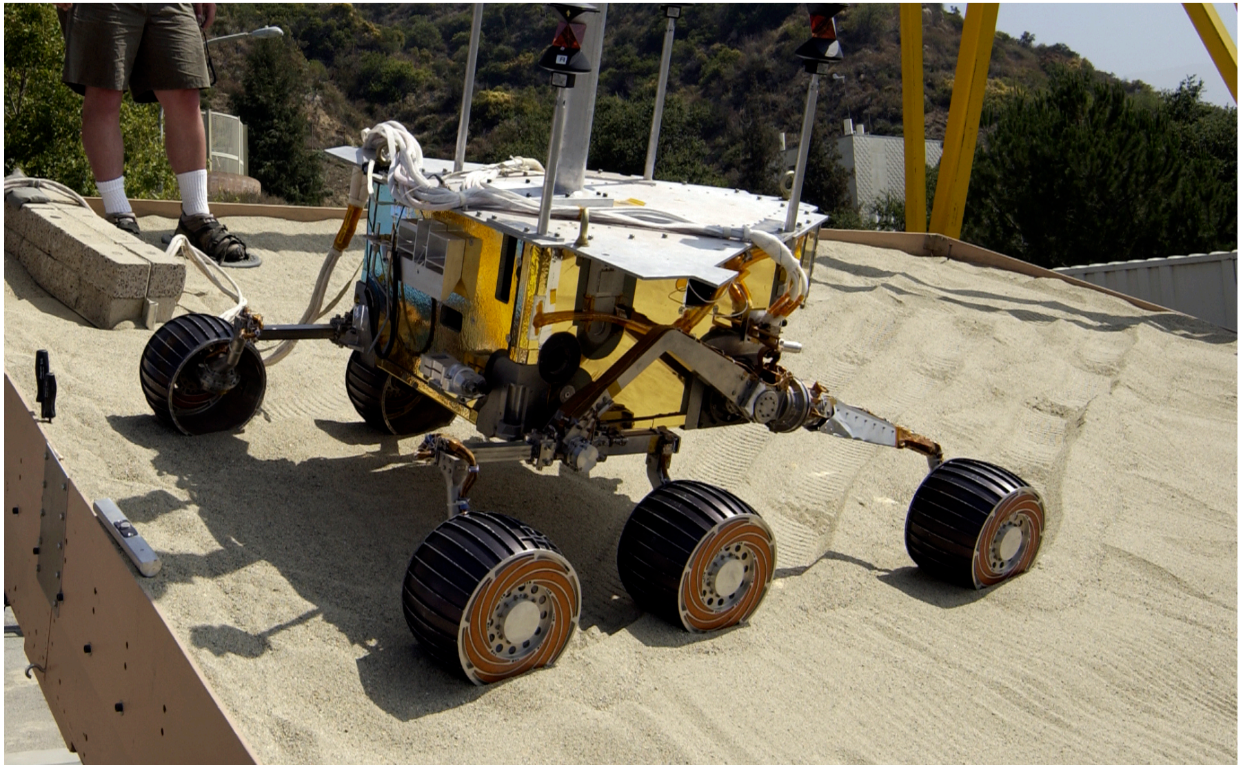
DTM Rover driving cross-slope on the VTTP, at a 20 deg slope, and covered with 20 cm of dry, loose quartz sand
