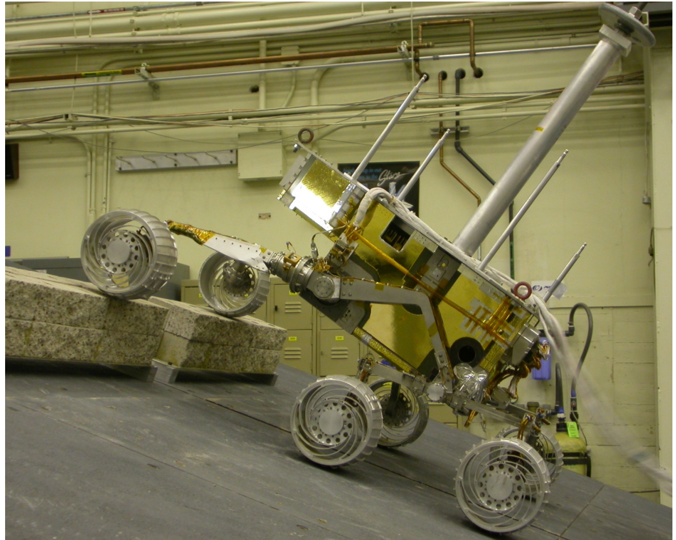
Dynamic Test Model rover driving up a 15 deg slope, climbing a 25 cm obstacle
