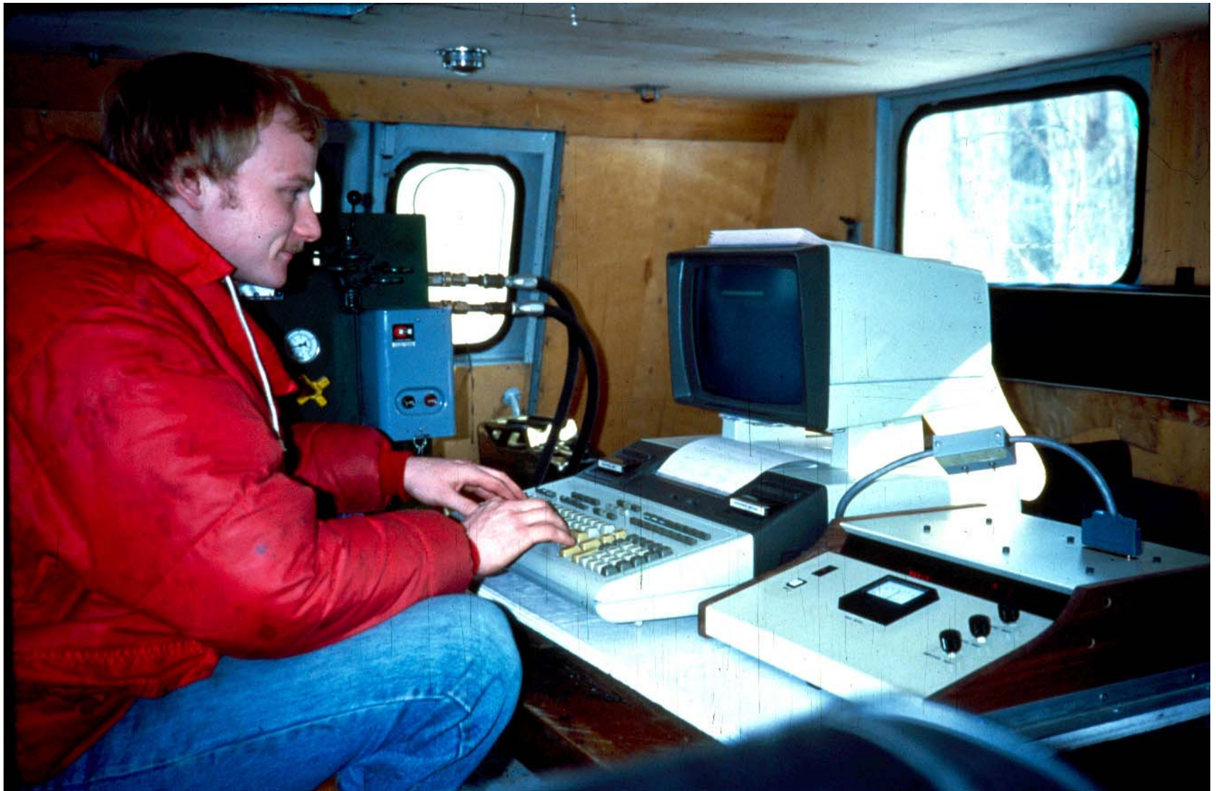
A computerized data processing system for a vehicle-mounted Bevameter.
