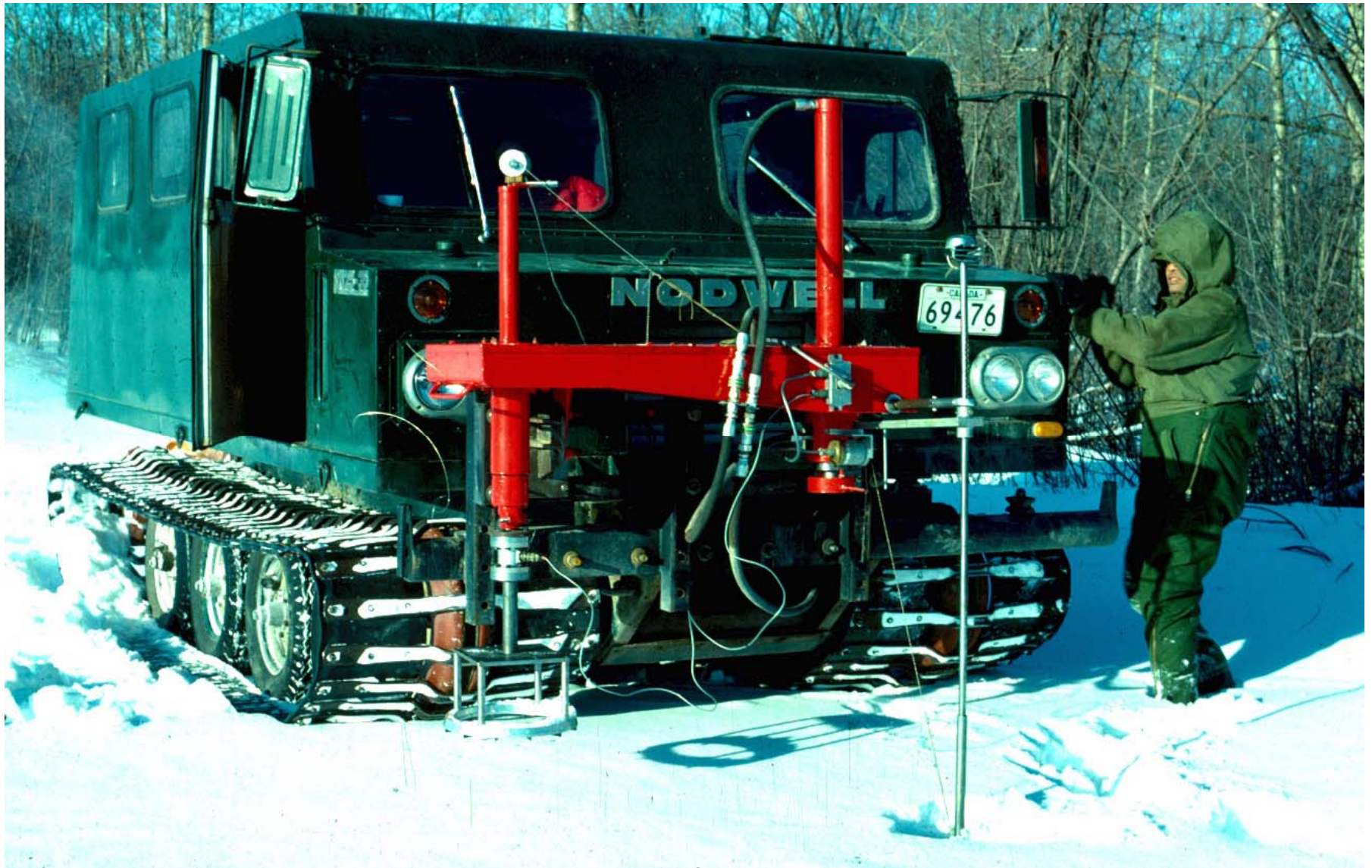
A vehicle-mounted Bevameter for measuring terrain properties.
