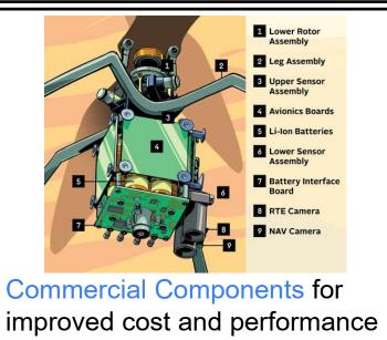
(Mars Helicopter electronics and sensors)
