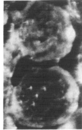
Sintering of two ice particles at -20°C. Sintering times: 3min, 1 day, 1 week
